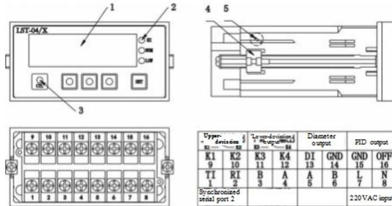
1. Display screen; 2. Alarm indicator lamp; 3. Input indicator lamp; put impedance of 100 Ω.
