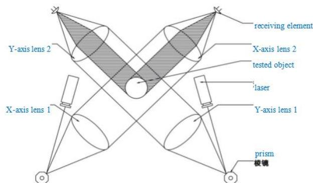
Fig. 2 (b) Two-axes Measurement Principle
