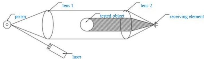
Fig. 2 (a) One-axis Measurement Principle
