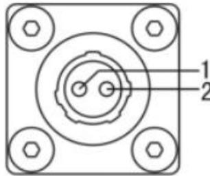
Power input port: 1 Pin: 24V input 2 Pin: Ground cable
